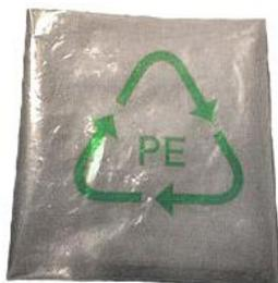
Ethylene is made by *cracking* natural gas or the light fractions of refined crude oil. It is converted to polythene by heat and pressure. A special substance called an *initiator* has to be added to get the *polymerisation reaction* started. Depending on the conditions, the polythene may have upwards of 10 thousand carbon atoms in each long chain molecule.
